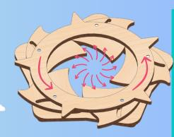
If you cannot rotate the mechanism freely, check if you leave enough clearance in STEP 3, else, undo STEP 3 and sand Part C more.
